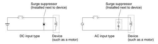
• If a surge suppressor does not fit on the device, installing a ferrite core directly next to the device's contactors, such as a contactor may be effective.
